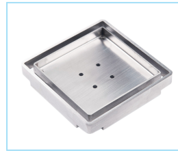
03 Premium tileable drain cover for Fundo Primo and Ligno: can be tiled with epoxy glue/adhesive or wedi Joint Sealant- used with 3/8 inch (9.5 mm) high tile or stone.
